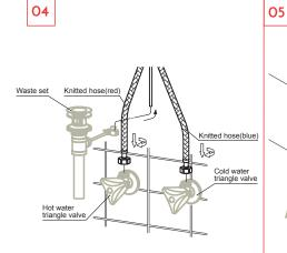
Connect the two knitted hoses to the two triangle valves (Red for hot water and blue for cold water). Connect the lower lift rod to the waste set.
