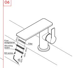
If the flow rate gradually decreases after sometime, it usually results from poor water quality leading to blockage of the filter. Please clean the filter as shown in figure above: Turn off the handle, unscrew the M3 screw with the S2 spanner, take off the mounting board, the flow straightener and the filterin turn, wash the filter and then install them back.
