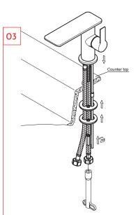
Pass the mixer body through the counter top, install the rubber washer and the mounting washer. Tighten them with the locking nut.
