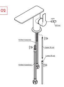
Connect the upper lift rod with the lower lift rod.Insert the lift nut into the slot on the back of the mixer body and connect it with the upper lift rod. Screw the knitted hose with red(hot) in front and bule(cold) in back.
