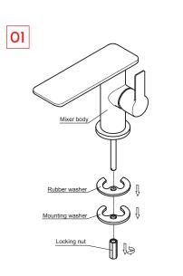
Disassemble the locking nut, mounting washer and rubber washer from the mixer body in turn.
